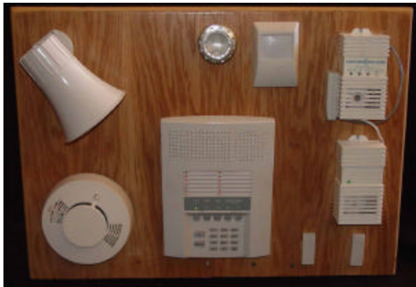
Photo 4. Interior alarm system showing system console, siren, smoke detector, motion detector, CO detector, Propane detector and two small magnetic switches
