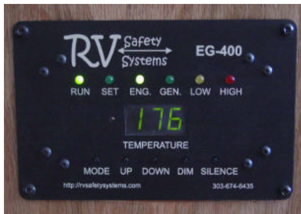
Photo 1. Engine and Generator Fire Detection system
