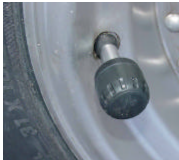
Photo 3. Tire pressure sensor mounted on valve stem.
